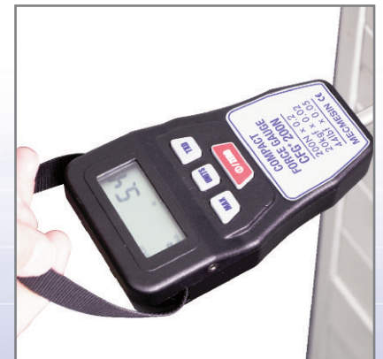
Tensile Test on Drawer
